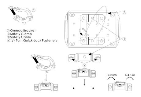
Regardless of the rigging option you choose for your LED moving head, always be sure to secure your fixture with a safety cable. The fixture providers a built-in rigging point for a safety cable on the hanging bracket as illustrated above. Be sure to only use the designated rigging point for the safety cable and never secure a safety cable to a carrying handle.
