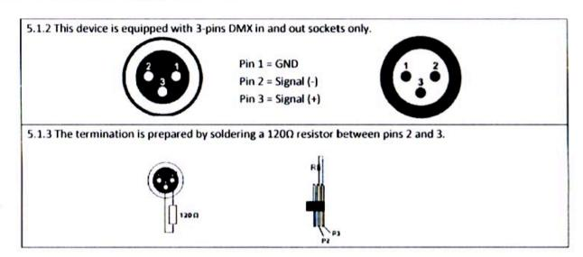
5.1.4 Connection: us DMX cable with 3-pin XLR-plugs to connect the controller with the fixture or one fixture with another.
